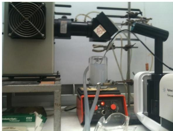
**Figure 1.** The Cary 60 UV-Vis fitted with the fiber optics microprobe accessory provides a simple mechanism to measure a sample *in situ* and remote to the instrument
